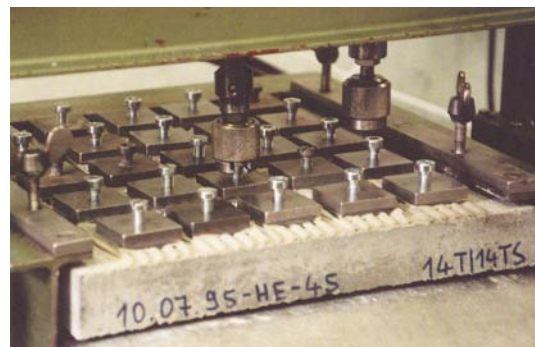
Equipment for testing tensile adhesion strength
